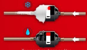
Temperature drops and/or frost or dew on the filter drier shell may indicate clogging and will require renewal of the filter
