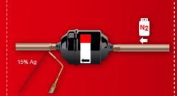
When brazing or welding, always apply N2 to the tubing while mounting
