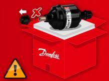
Keep the filter drier seals in place at all times and do not break the seals before the last moment before mounting!
